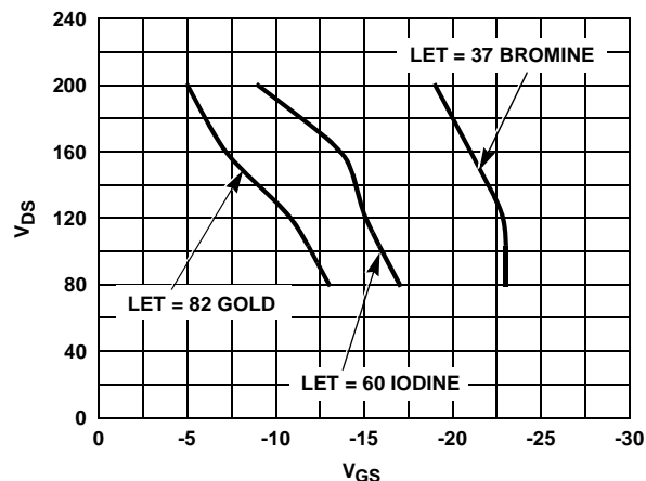
FIGURE 2. TYPICAL SEE SIGNATURE CURVE
